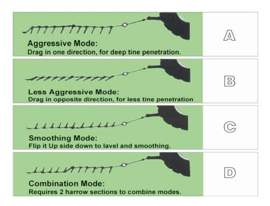
1. Lay Down All sections Of Chain Harrow Wide Open With Tines Touching The Ground As Shown In The Picture **A**.
